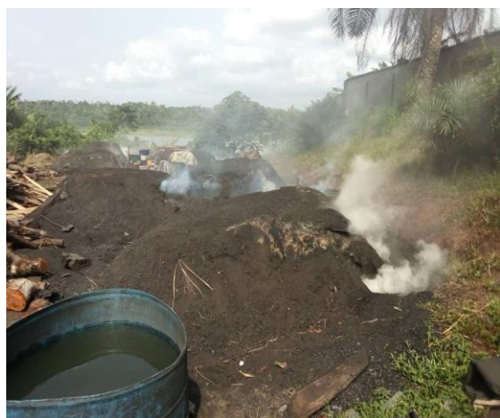
Plate 4: A kiln with a drum of water for controlling the rate of burning logs
